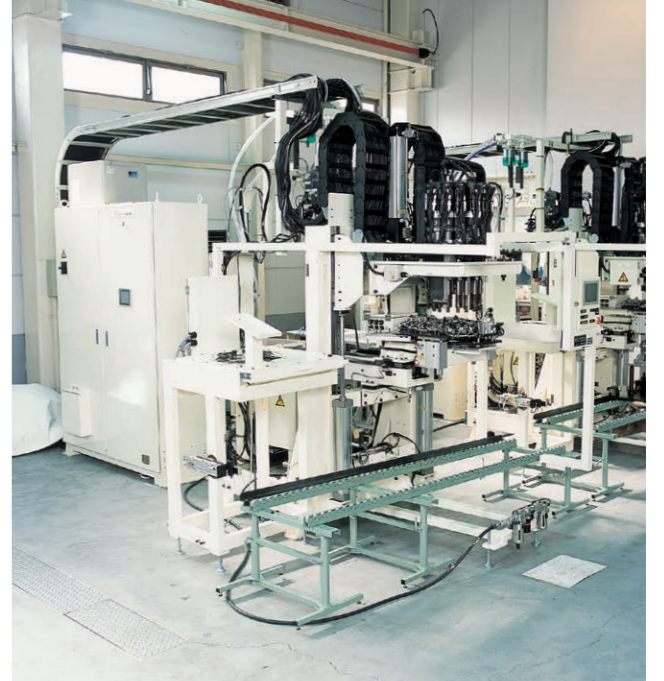
Side Cover Fastening Machine with Automatic Bolt Feeder
